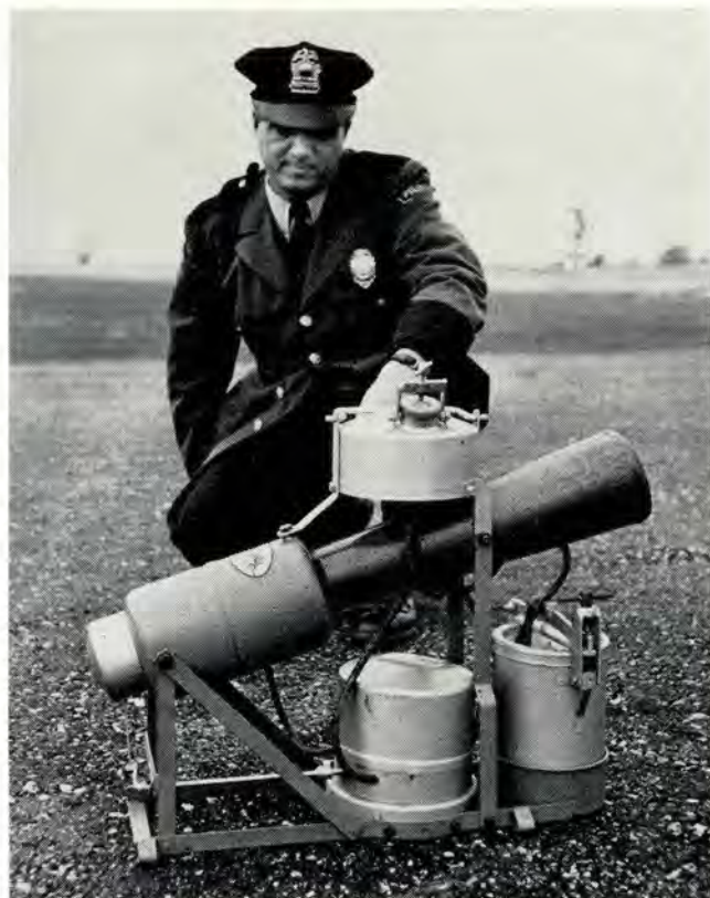
Bird scare devices at Washington National Airport (above) and Idlewild International (below, right) are being tested in war against feathered threat to aircraft. Jet engines are particularly vulnerable to bird ingestion.
